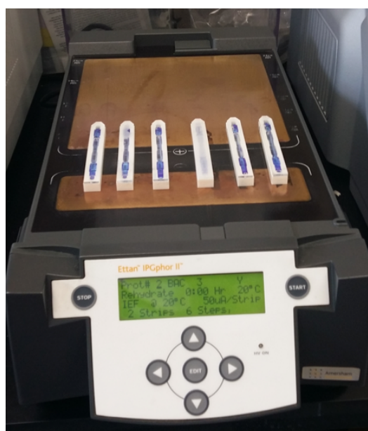
Figure 2.1 Isoelectric focusing Ettan IPGphor II used in 2D IEF SDS-PAGE
