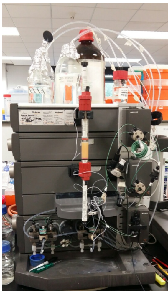
Figure 2.4 ÄKTA-FPLC with attached column containing Q-Sepharose™ beads and B. oleronius protein sample
