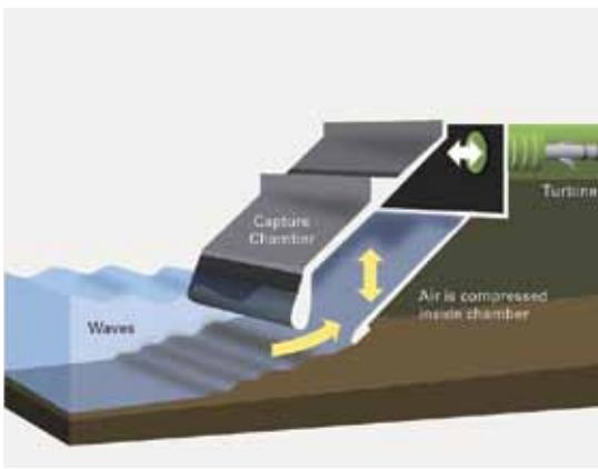
Figure 5: Oscillating water column principle of operation.
