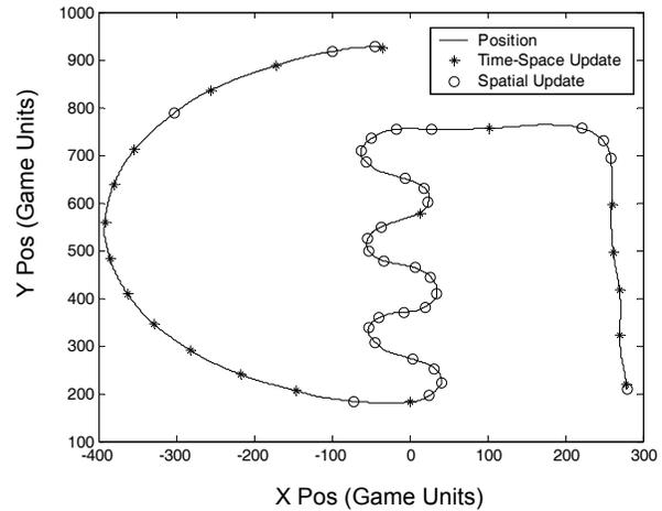
Figure 4 – Varying updates are transmitted as the curvature of the course changes
