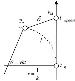
Figure 1. Actual and dead reckoning model position
