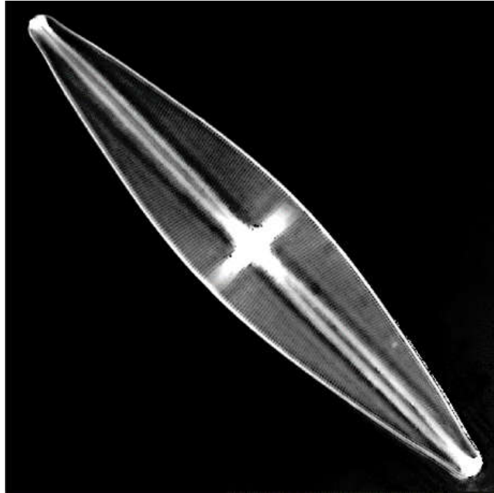
Figure A.2: The phase image of the diatom cell reconstructed from the SA hologram before using deconvolution algorithm
