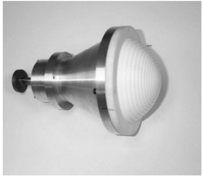
Figure 2 Horn plus lens at 30 GHz
