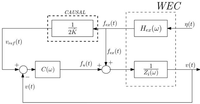
FIGURE 7 – Real-time implementation of reactive control as a velocity-following. If system model is  $2^{nd}$ -order, reference generation is a purely proportional block, which is *causal* and realisable.
