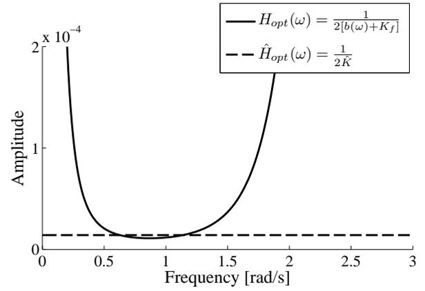
FIGURE 6 – Velocity-generation law,  $V(\omega)/F_{ex}(\omega)$ , for reactive control calculated for full system and  $2^{nd}$  order approximation model (constant over frequency). The system is cylinder 2 of Table 1.
