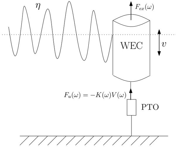
FIGURE 1 – Floating cylinder constrained to move in the heaving direction. The PTO force,  $f_u$ , is assumed to be related to the velocity through a law of the type in Eq. 6.
