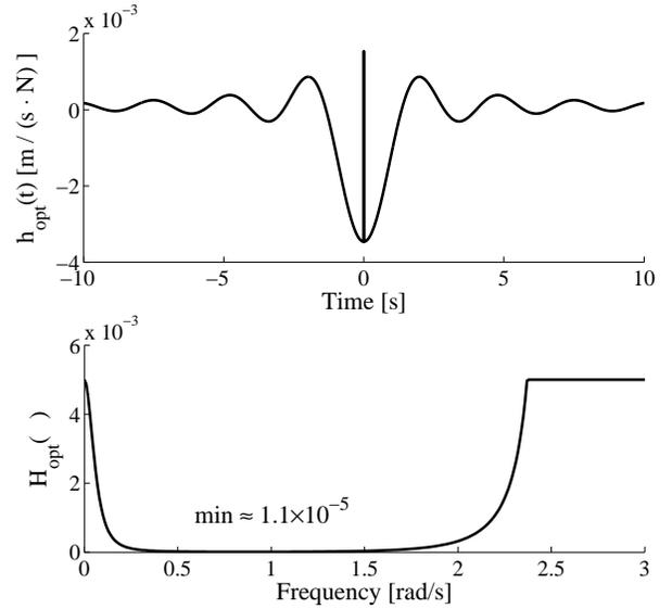
FIGURE 3 – Non-causal transfer function between excitation force and optimal velocity. Example for a heaving cylinder of radius  $R = 5m$ , draught  $h = 6m$  and submerged mass  $M = 3.9 \times 10^5 Kg$ .
