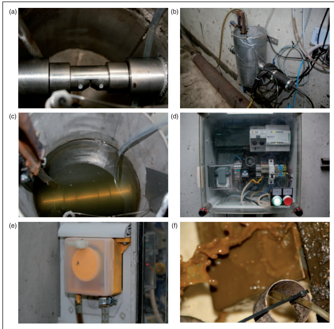
Figure 3 (a) UV/vis-probe with 1 mm gap width; (b) complete layout of the measurement system; (c) online-measurement in progress; (d) control cabinet for the measurement system; (e) flexible-tube pump for exact dosing of the fermentation sludge; (f) collection container for the press water of the fermentation sludge.
