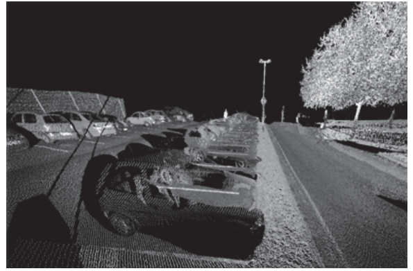
Figure 3: An example of a MMS Point Cloud
