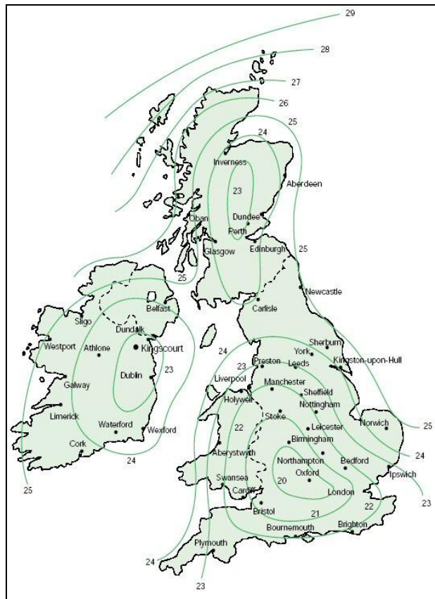
Figure 5.2 10-minute-mean wind speed with a 1:50 year risk of exceedance (m/s). (Source: Kingspan, 2012).
