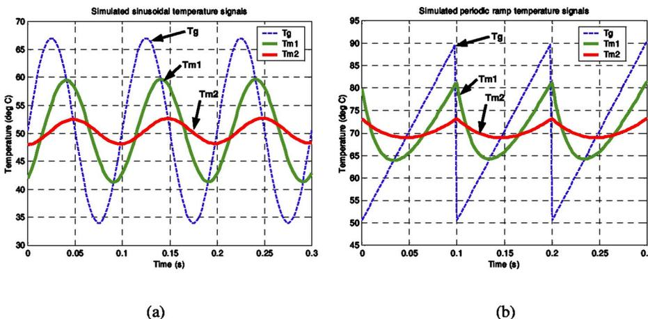
FIG. 3. (Color online) Simulated (a) sinusoidal and (b) periodic ramp gas temperatures and the corresponding thermocouple outputs (time constants are 0.0238 and 0.1168 s, respectively).
