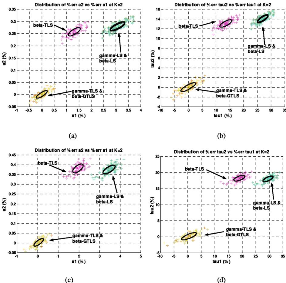
FIG. 5. (Color online) Distribution of percentage errors of  $\hat{a}_2$  vs  $\hat{a}_1$  [Eq. (23)] and  $\hat{\tau}_2$  vs  $\hat{\tau}_1$  from different algorithms at noise level  $K=2$  for (a) and (b) sinusoidal and for (c) and (d) ramp signals, respectively. TDR-Kee distributions were outside the range and are thus omitted.
