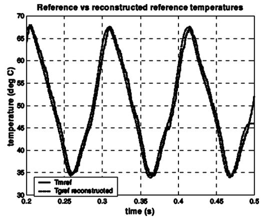
FIG. 9. Recorded  $T_{mref}$  and reconstructed  $\hat{T}_{gref}$  reference thermocouple ( $\hat{\tau}_{ref}=0.0026$  s) temperature signals. It is evident that due to the very small time constant, attenuation of  $T_{mref}$  is negligible.
