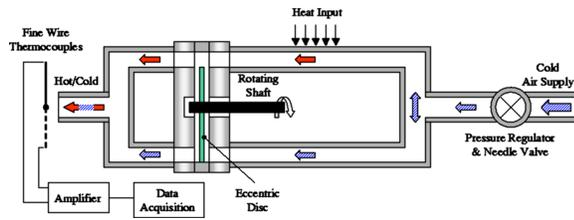
FIG. 8. (Color online) Schematic illustration of test rig.
