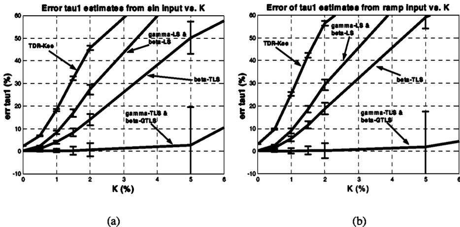
FIG. 4. Mean and standard deviation of percentage errors of  $e_{\tau 1}$  against noise relative to signal  $K$  from (a) sinusoidal and (b) ramp signals, respectively.
