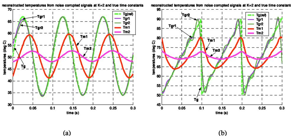
FIG. 7. (Color online) Portions of postfiltered (a) sinusoidal and (b) periodic ramp temperature reconstructions from noise-corrupted thermocouple outputs at  $K=2$  and true time constants. The filter bandwidths are (a) 20 and (b) 50 Hz, respectively.
