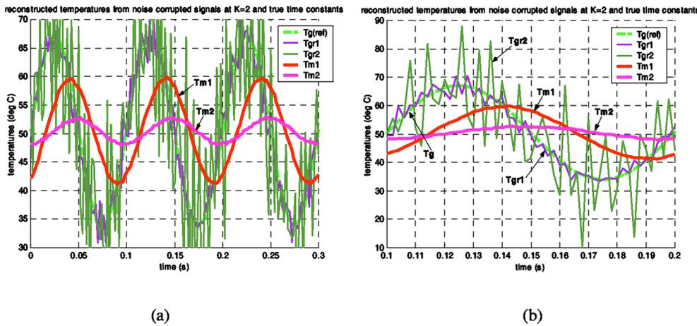
FIG. 6. (Color online) Sinusoidal temperature reconstructions from noise corrupted thermocouple outputs at  $K=2$  and true time constant; (b) is a close-up version of (a) between 0.1 and 0.2 s. “Tgr1” and “Tgr2” are the reconstructions from thermocouple outputs 1 and 2, respectively.
