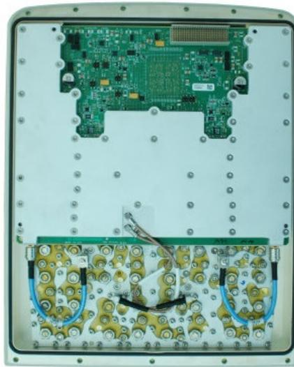
**Figure 2.8:** A typical metrocell base station with back case removed [5].
