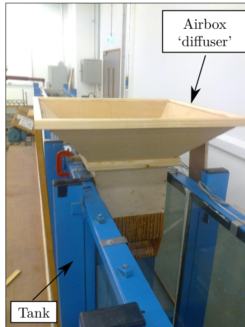
FIGURE 10.4: Model 2 installed in tank prior to the final stage of model construction, during which the large airbox was installed.
