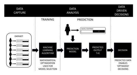
Figure 3 The data capture, analysis and decision cycle enabled by predictive AI
