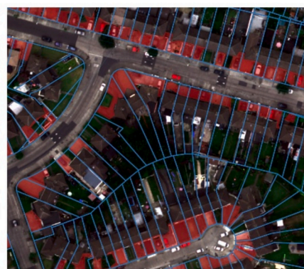
Fig. 5. Potential driveways (in red) detected in the test area. (For interpretation of the references to colour in this figure legend, the reader is referred to the web version of this article.)
