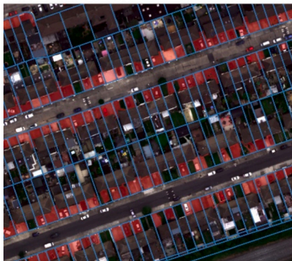
Fig. 5. Potential driveways (in red) detected in the test area. (For interpretation of the references to colour in this figure legend, the reader is referred to the web version of this article.)
