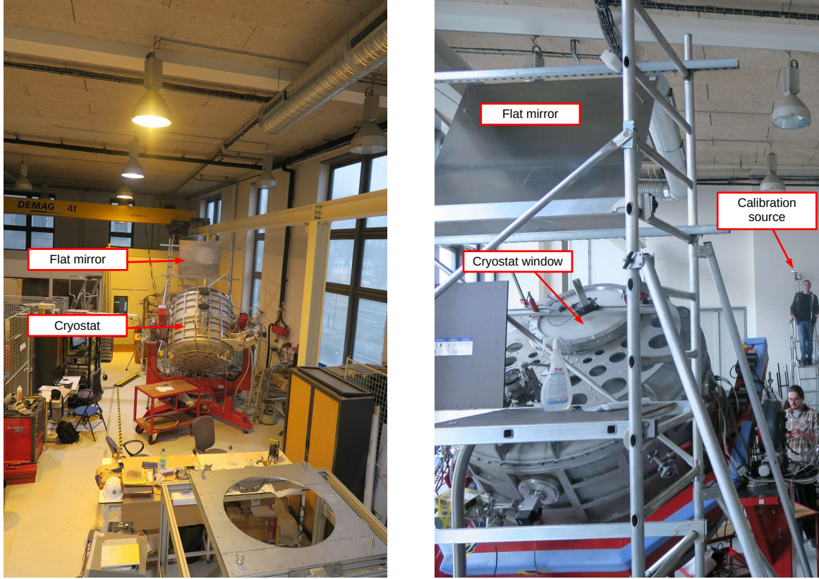
Figure 3. Left: photo of QUBIC looking along the line-of-sight from the calibration source. The reflection of the window is clearly visible in the flat mirror. Right: the flat mirror is mounted on a scaffold at a height of 3.7 m and has a finely adjustable tilt angle using a system composed of a long screw.
