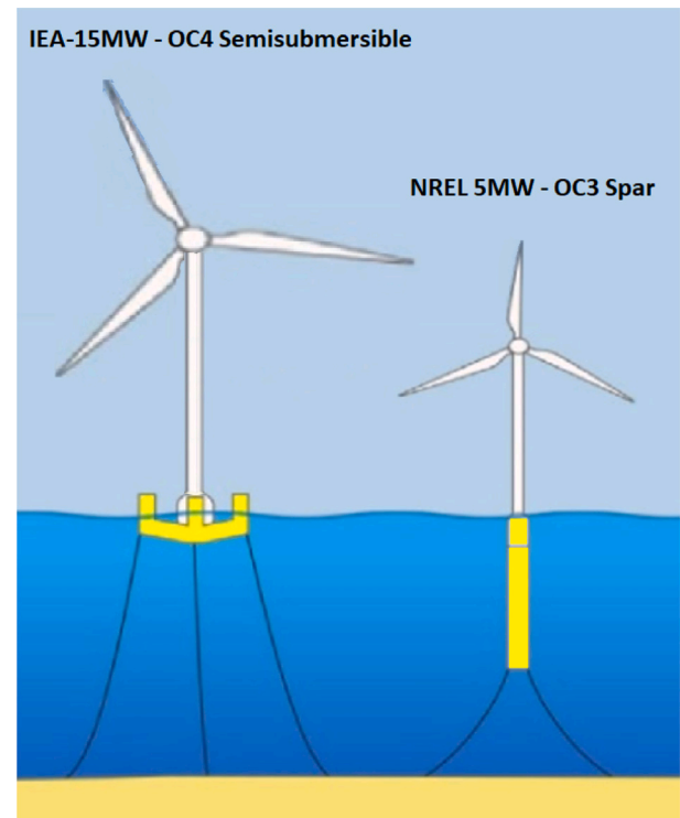
Fig. 4. Sketch of the floating turbines used in the analysis (Shafiee, 2023). (Notably, the dimensions are approximate and do not represent the real scale).
