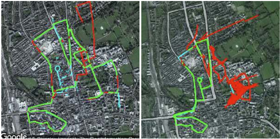
Figure 1.5: Left: Mapping error (red) caused by poor GPS reception in Oxford, where raw GPS values are shown in cyan. Right: A loss of reception causing significant positioning error over a large portion of the route [7]. Best viewed zoomed in colour on a computer screen.
