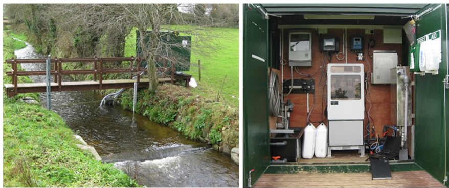
Fig. 4 High-frequency water quality and hydrometric monitoring station within the Irish Agricultural Catchments Programme. This setup monitors concentrations of total reactive phosphorus, total phosphorus, total oxygenated nitrogen, total organic carbon and suspended sediments (derived from turbidity) together with electrical conductivity, temperature and river discharge (derived from river stage). All data is collected at a sub-hourly resolution since 2009. This shows that high-frequency monitoring requires a robust setup for long-term monitoring
