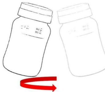
Figure 2 Swirl agitation indicative illustration
