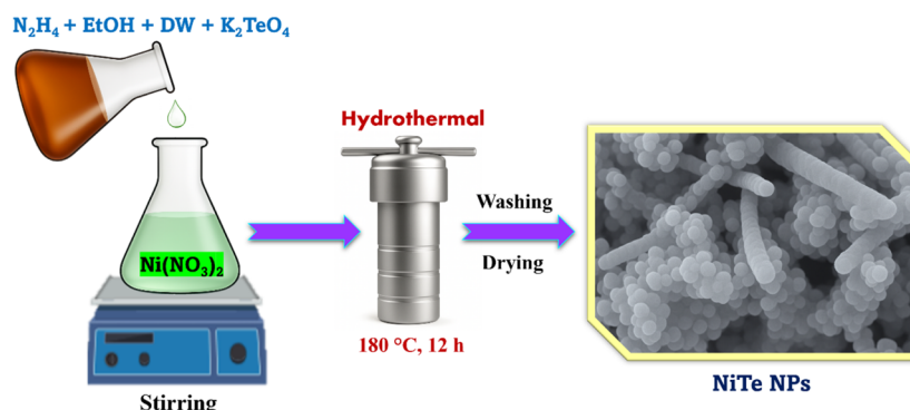
Figure 1. Schematic illustration of the hydrothermal synthesis of nickel telluride nanoparticles (NiTe NPs).
