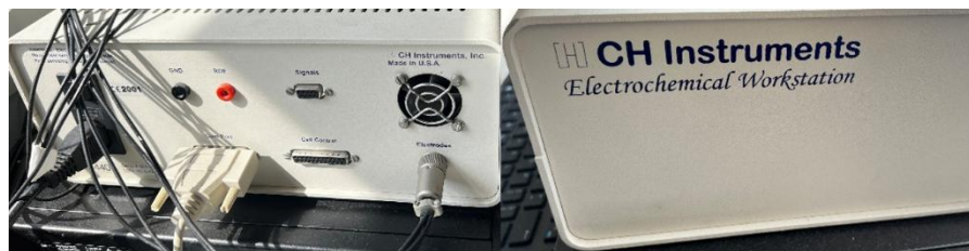
Figure. 2.8. The CHI440 CH Instruments, Inc. potentiostat for used in the differential pulse voltammetry (DPV) analyses.
