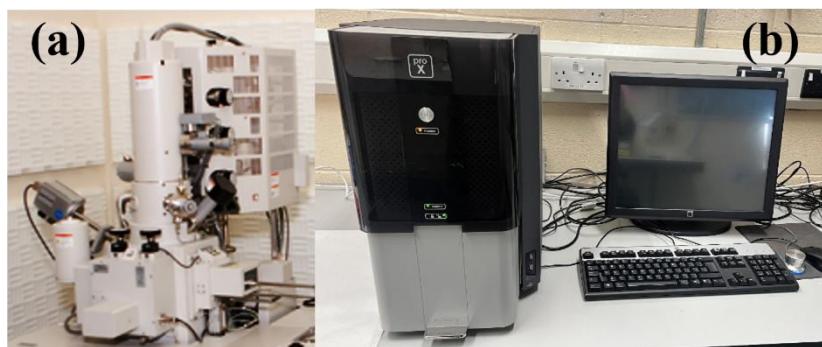
Figure. 2.11. (a) Hitachi S-4800 FESEM was used in Chapters 3-5, and (b) SEM phenom world pro X was used in Chapters 6-7 of the SEM studies.
