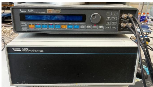
Figure 2.10. A Solartron 1287 potentiostat coupled with a 1250 or 1255 FRA (Solartron) electrochemical impedance spectroscopy (EIS).
