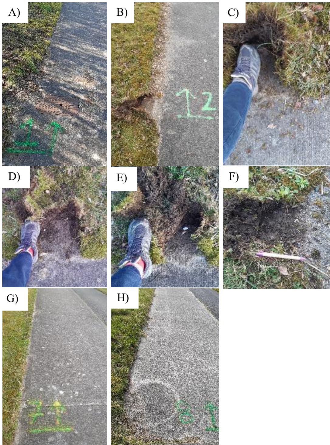
Plate 5-4 The effect of treatments along the grass verge. Control (A), Hot Foam (B), Roundup Flex (C), Nomix Dual (D), Strim/Mow (E) and New Way (F) had no impact on the grass verge eleven months post-treatment. The WeedHex machine (G) and the Multihogg machine (H) had little impact on the intersection but cleared the grass verge completely. The grass verge was still cleared of soil after both mechanical treatments, but vegetation was beginning to encroach from the grass verges, by the final survey eleven months later.
