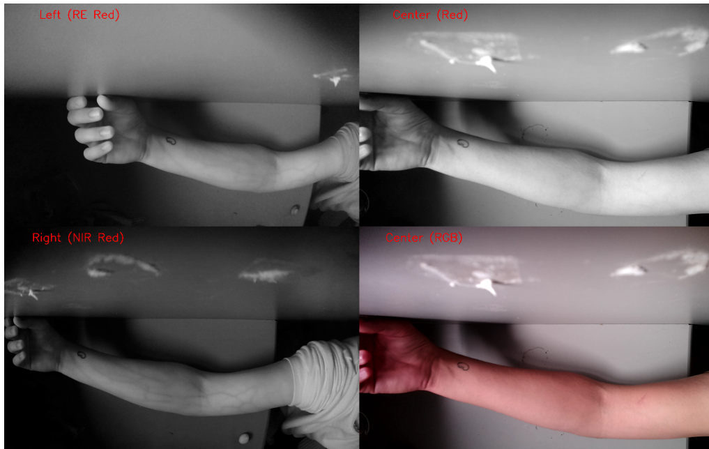
Figure 5.2: a) RE image showing visible veins, b) VIS red image showing barely visible veins, c) NIR image showing very clearly visible veins, d) RGB image showing almost no veins
