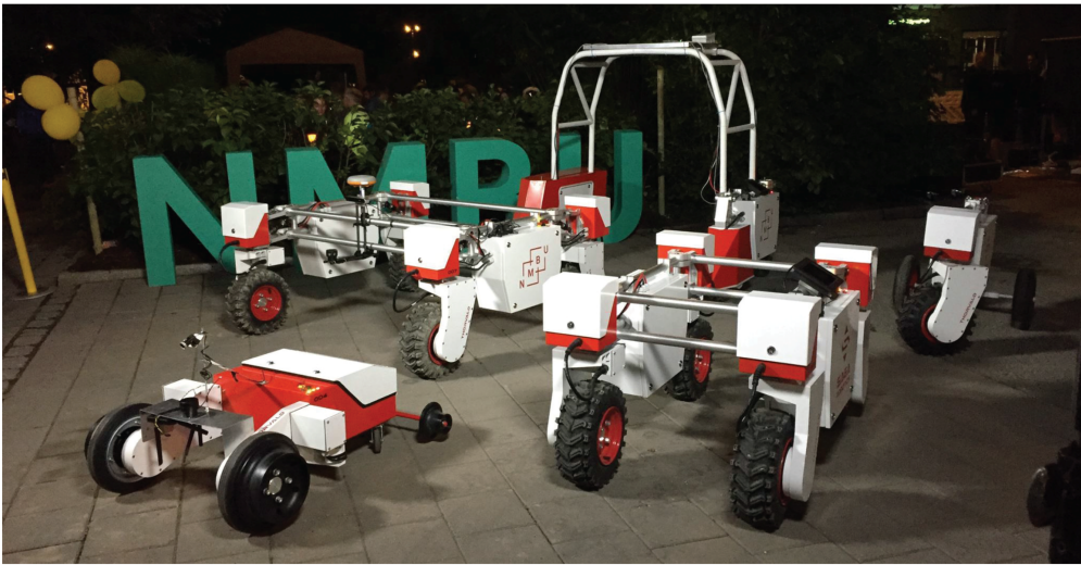
Figure 2.2: The Thorvald II Agricultural Robotic System
