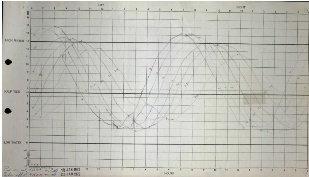
Figure 4.2: Example of a Cork marigram with a pencil trace. The X-axis represents time from 06:00 am–06:00 am the following day, and the Y-axis shows water level in feet relative to chart datum. Dates are indicated above the pencil traces. Data courtesy of Port of Cork engineers (personal communication, 2022).
