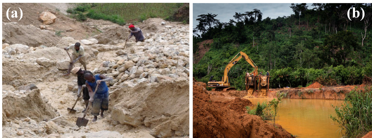
Figure 1.1: Typical ASM operations. (a) Artisanal coltan mining, ground sluicing using simple tools such as picks and shovels in Rwanda (source: Dorner et al., 2012 ). (b) Artisanal gold mining employing heavy machinery such as an excavator in the wet tropical forest in Ghana (source: Bansah et al., 2018 ).
