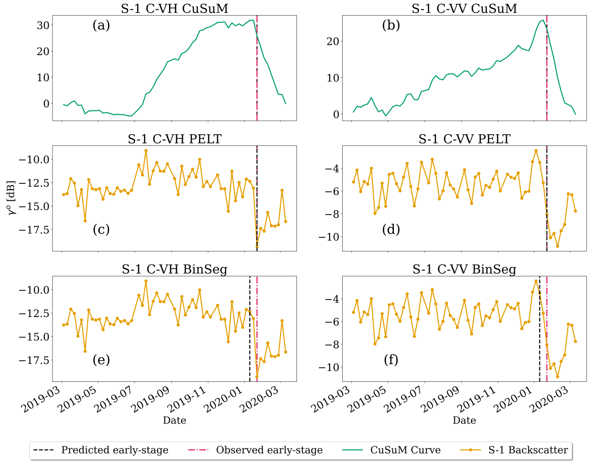
Figure A8: Intact forest (left) and ASM-induced deforested (right) smoothed S1 backscatter time series over mine site 5 in the Western test site for both C-VV and C-VH polarisations. Structural changes due to the start of ASM activity detected using CuSuM, PELT, and BinSeg algorithms are presented (vertical lines). The change (early stage) is shown in the next observation in the time series (dotted black line). The date from optical NDVI (dotted red line) was used as validation.
