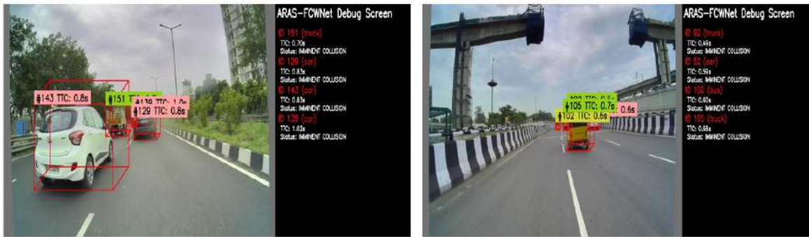
Figure 6: ARAS-FCWNet Debug Screen Status: Imminent Collision using TTC Performance
