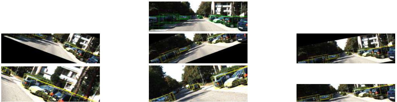
Figure 4: DED Generality on KITTI. We apply DED to KITTI to demonstrate the generality of our augmentation. (Top) Original image. (Middle) Warped images showing perspective distortion. (Bottom) Final cropped images with transformed ground truth. This creates a challenging benchmark for geometric robustness on standard automotive data.
