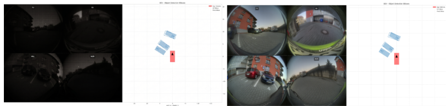
Figure 4: BEV-space detection inference using BevFormer in real 16-bit Bayer RAW and ISP processed Image in automotive fisheye imagery dataset. The left side shows inference on RAW image and right side shows inference on ISP processed image
