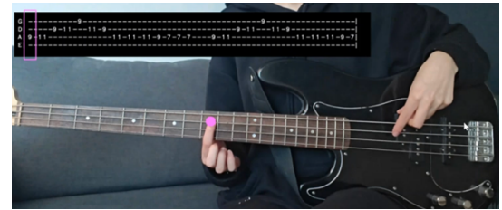
Figure 5: The system interface showing the tablature (top) and a live video feed of the guitar with a pink dot highlighting the string/fret to be played
