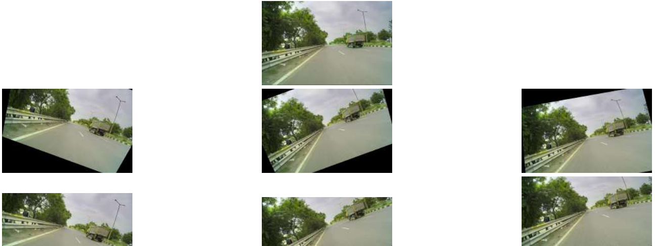
Figure 3: DED on our ARAS Dataset. (Top) Original image and 3D box. (Middle) Warped images for different drift parameters. (Bottom) Final cropped images. Our method applies the same 3D rotation to the ground truth, producing new, physically-correct labels for the augmented views. Drifts (L-R): (R:+20°, P:+10°), (R:-20°, P:+5°), (R:-10°, P:-5°).
