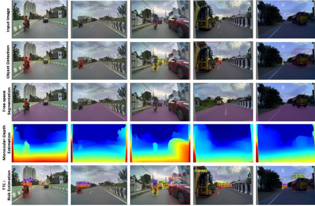
Figure 4: ARAS-FCWNet Multi-Task Perception Network: (i) Object Detection, (ii) Free-space Segmentation, (iii) Monocular-Depth Estimation, and (iv) TTC-based Risk Estimation.
