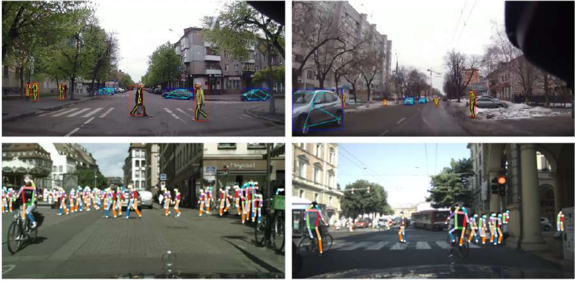
Figure 4: Examples of semantic keypoint detection for pedestrians and vehicles using OpenPifPaf on JAAD and BDD100K datasets.
