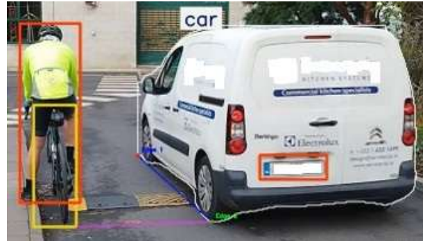
Figure 1: The bicycle (yellow box), cyclist (red box), passing vehicle (white outline), and licence plate (orange box) are all located using YOLO. The distance from the vehicle’s wheel to the bicycle/person is measured (purple line) in pixels and converted to centimetres using the size of the licence plate
