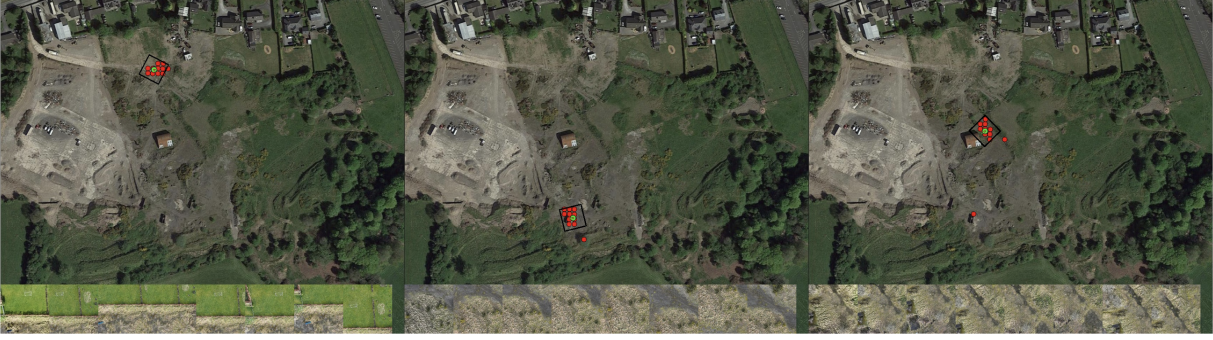
Figure 4.9: Examples of the IBL system successfully estimating the location of the UAV. The green particle shows the ground truth of the UAV, and the red show the top 10 position estimates.
