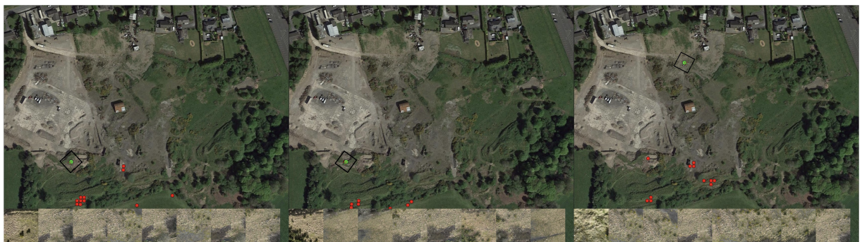
Figure 4.11: Examples of failure in estimating position due to ambiguous vegetation present in a rural scene. The green particle shows the ground truth of the UAV, and the red show the top 10 position estimates.
