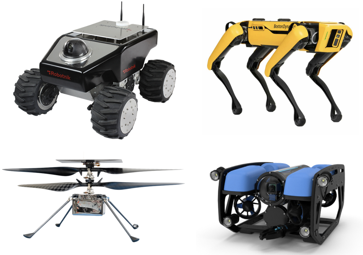
Figure 1.1: Examples of different robot configurations: Wheeled (top left) [132], Gating (top right) [17], Flying (bottom left) [98] and Marine (bottom right) [4]
