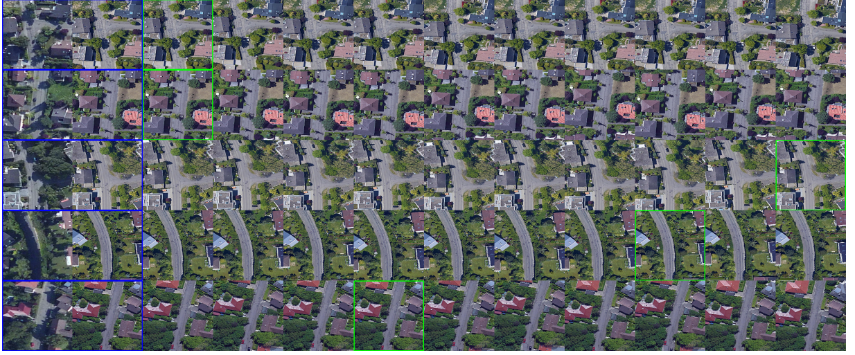
Figure 4.8: Example of successful aerial images queries in a cross-time urban environment. The green box depicts the correct match and in blue the ground truth pair. Data Attribution: Imagery 2023 CNES / Airbus, GeoBasis-DE/BKG, GeoContent, MaxarTechnologies, Maps Data: 2023 Google.
