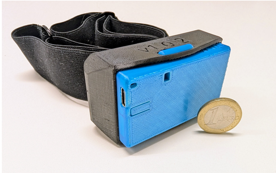
Figure 3.31: Isometric view of Prototype #3 in comparison with a €1 coin, showing the small size and minimalist design.
