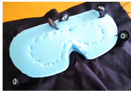
(f) Rear view of memory foam for eye sockets with the snap-fastener connections coming through or around the foam.
