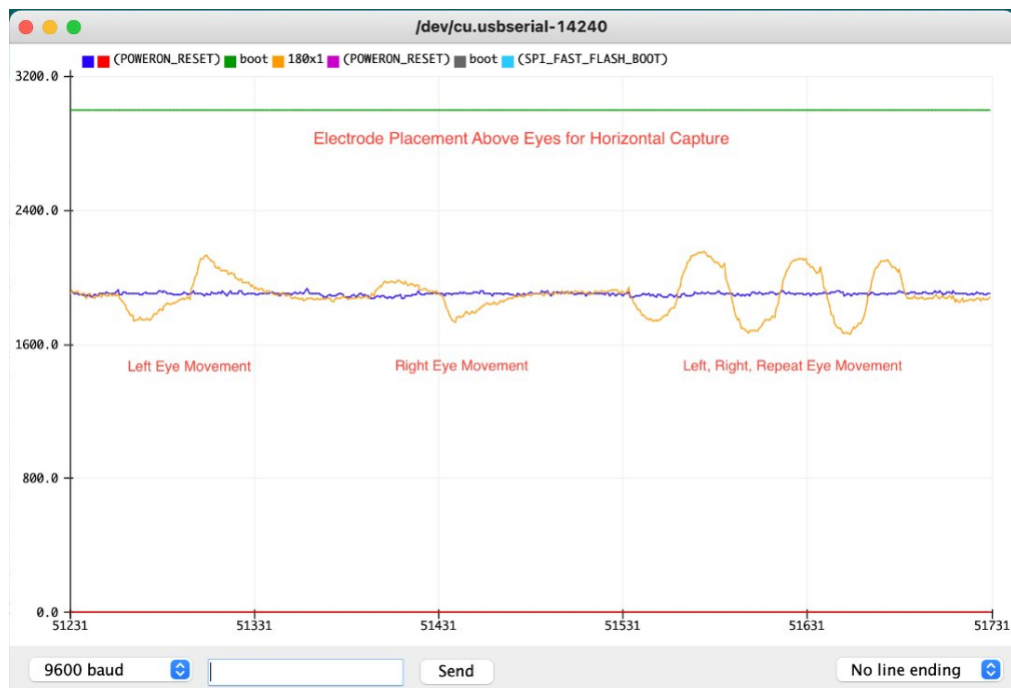
Figure 3.14: Recording of Placement 1. Eyebrow placement produced signal amplitudes approximately half those obtained from lateral placements. Green line shows maximum potential value, yellow line is measured AD8232 values, blue line is unused, second AD8232 input.
