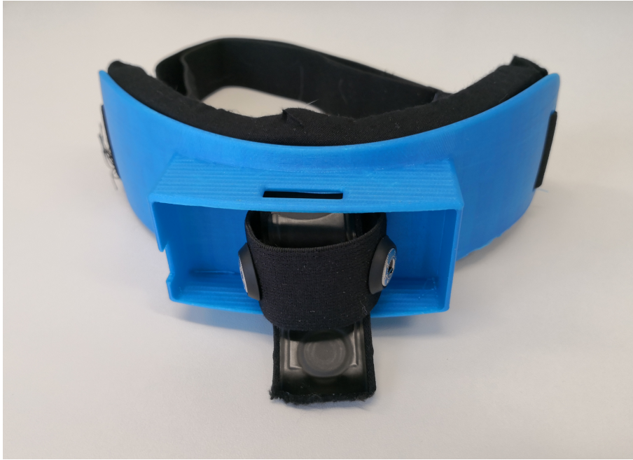
Figure 3.26: Early Version of Prototype #2, featuring a PLA printed chassis, Lyocell wrapped memory foam support, and 1.5 HRMCS. This image shows the snap electrode connections of the HRMCS tucked within the electronic case slot, indicating how the tertiary electrode strap folds around the main, horizontal HRMCS.
