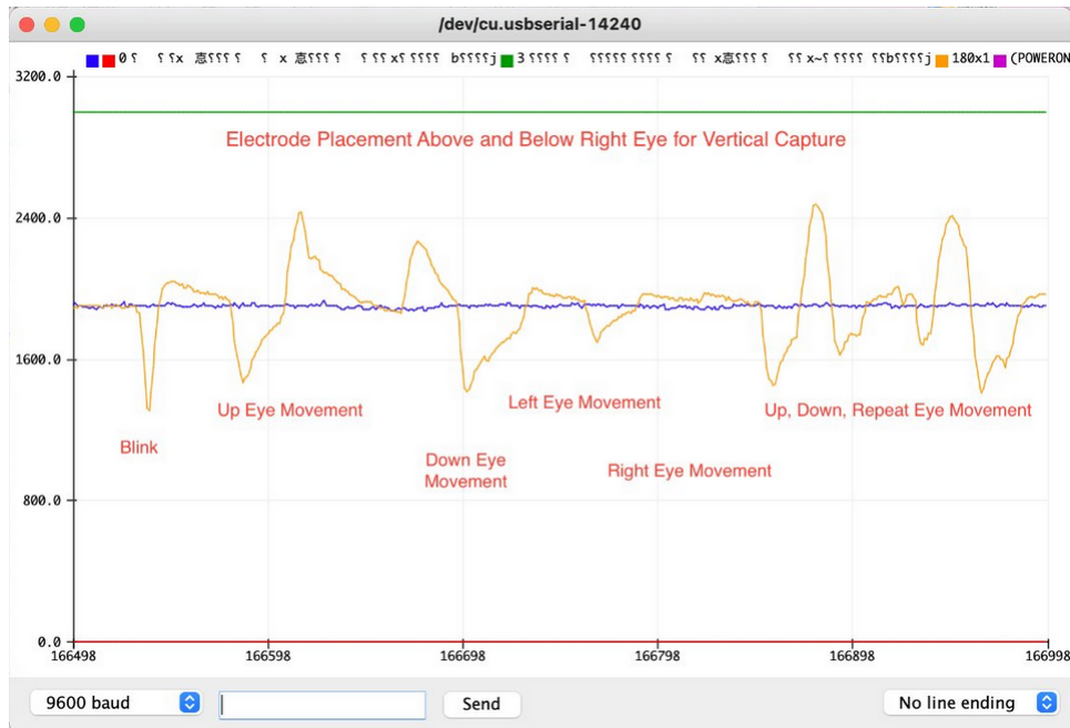
Figure 3.12: Recording of Placement 3 (above and below the right eye). Sequence: blink, followed by up, down, left, and right eye movements, then sustained up-down repetition. Green line shows maximum potential value, yellow line is measured AD8232 values, blue line is unused, second AD8232 input.
