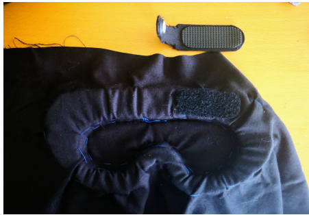
(e) Padded eye socket with a soft loop patch above the right eye position, and hook patch attached to rear of CTPU electrode.
