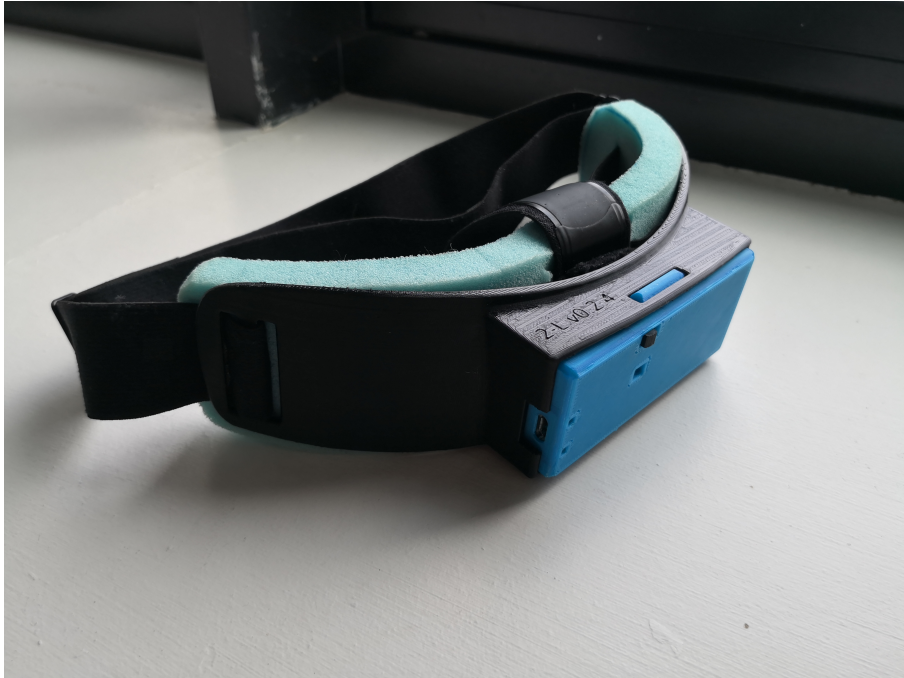
Figure 3.25: Isometric view of Prototype #2 showing the headband design with integrated electronic case. The electronic case, in blue, is printed with PLA and the receiver, in black, in TPU-95. Visible on the front of the electronic case is the microphone window, and the new locking tabs to secure the case to the receiver.
