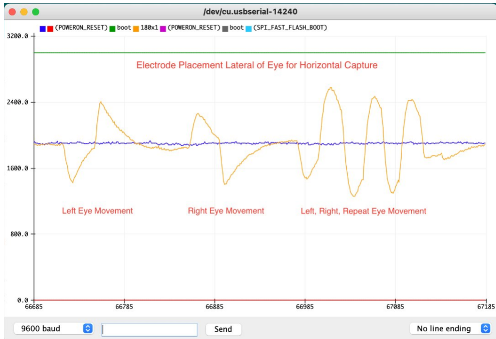
Figure 3.13: Recording of Placement 2 (lateral to each eye). Green line shows maximum potential value, yellow line is measured AD8232 values, blue line is unused, second AD8232 input.
