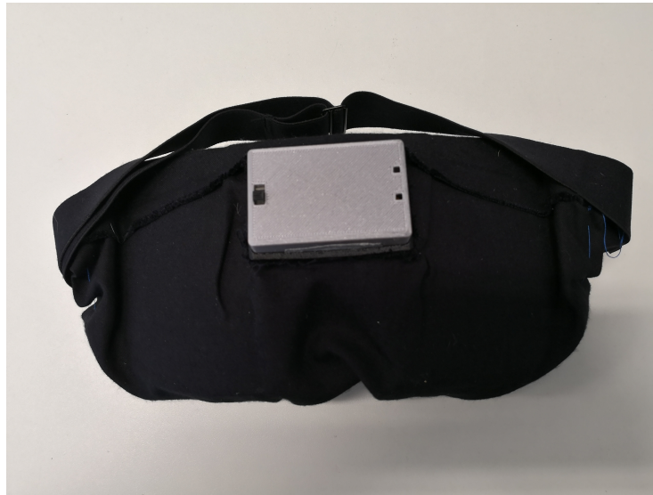
Figure 3.18: Front view of Prototype #1 (MVP) showing the sleep mask form factor with integrated electronics housing (in silver PLA) and a Lyocell fabric covering. Visible are the ON/OFF switch and two windows in the electronic case for LED notifications.
