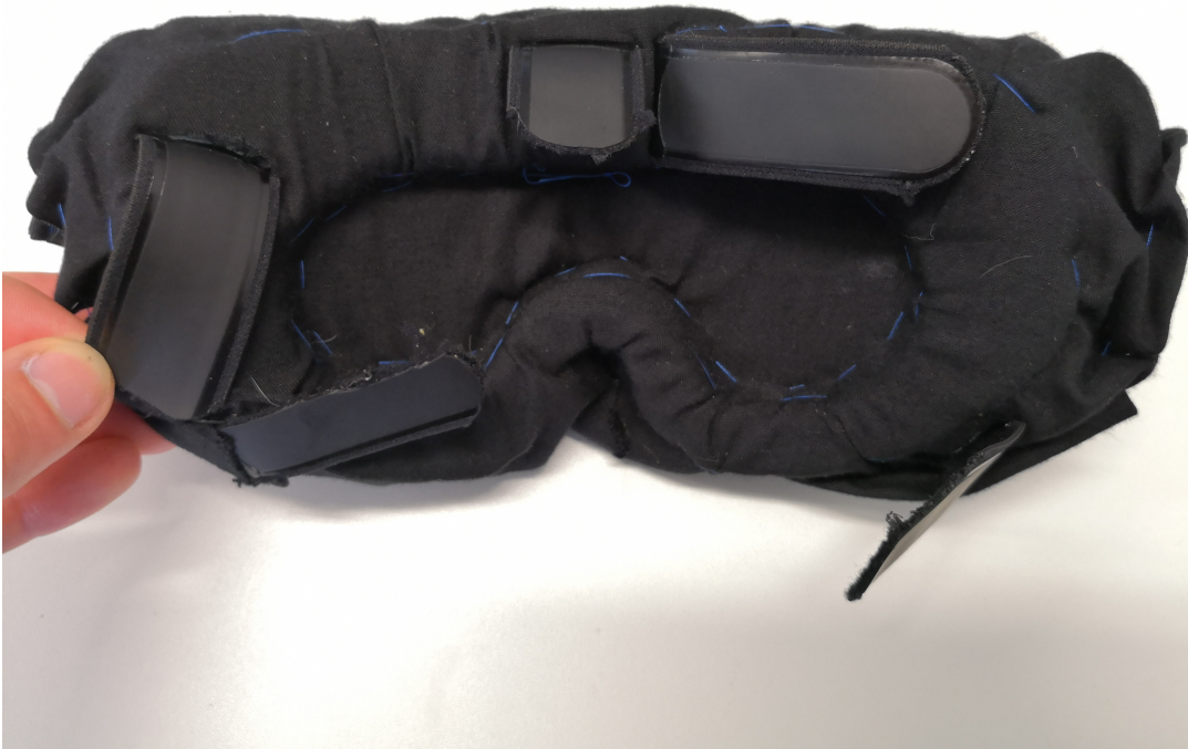
Figure 3.24: Rear view of Prototype #1 showing memory foam padding and electrode positioning for comprehensive EOG coverage. This image was from 1 month after construction, and demonstrates the poor reliability of the Velcro adhesive to the Lyocell fabric.
