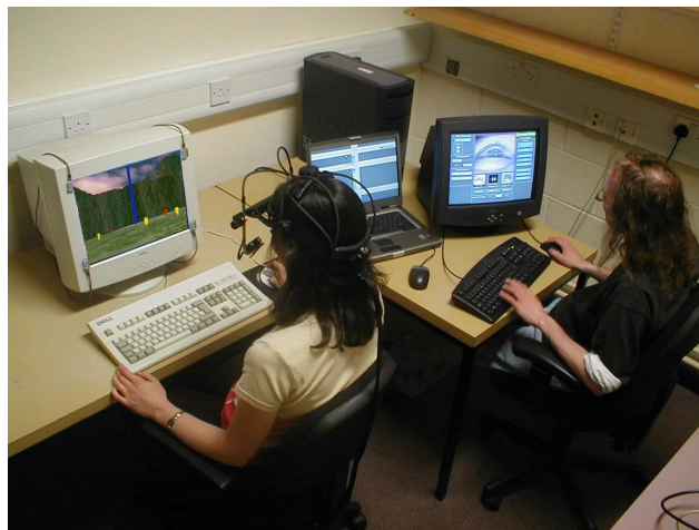
Figure 3: Experimental setting with the SR Research EyeLink II eye-tracking system in the laboratory.
