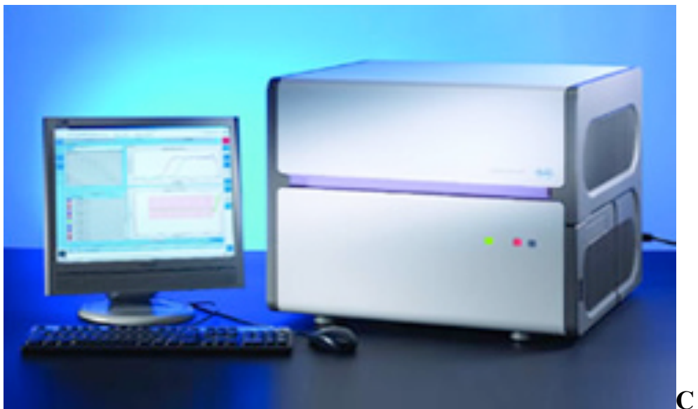
Figure 2.3 (A) G. mellonella RNA on a 1% agarose gel visualized under UV light (B) The intercalation of SYBR Green with DNA and the fluorescent emission (Section 2.8.1) (C) Roche ® Light Cycler 480 used in this work for Real Time PCR (Section 2.8.1)
