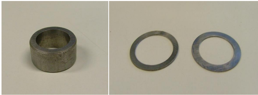
(a) (b) Figure 4.15 (a) A single cylinder, that mimicks the effects of adding a thick plate was placed in front of a corrugated horn. (b) Two examples of the rings used to measure the effects of adding a corrugated block in front of a corrugated horn.
