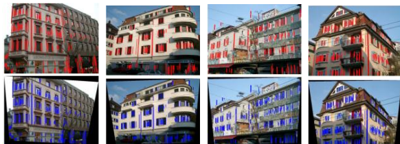
Figure 1: Some example results of camera tilt rectification (top row: original images, bottom row: rectified images). The vertical edges are highlighted to demonstrate the effect.
