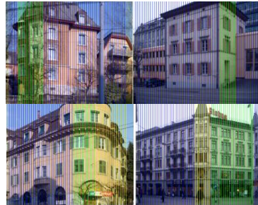
Figure 5: Some examples of 3D reconstruction. The color-coded vertical strips correspond to 3D planes in different directions
