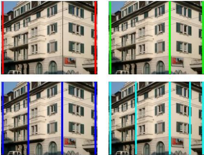
Figure 3: The process of generating piecewise planar 3D building layout candidates by adding more vertical lines into the existing models.
